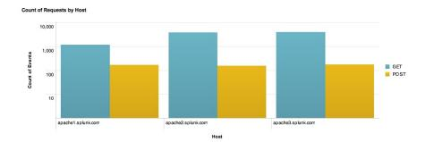
This chart displays the total count of events for each event type, GET or POST, based on the host value. The logarithmic scale is used for the y-axis because of the difference in range of vales between the number of GET and POST events.
